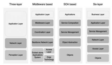
Figure 4. IoT Layered architecture.
