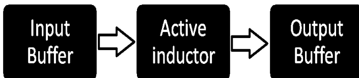
Fig. 5. Block diagram of the proposed inductor-less Band pass filter.
