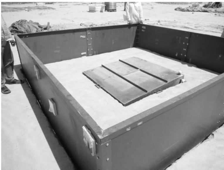
**Fig. 4.** Set up of SDRI device in the field.
