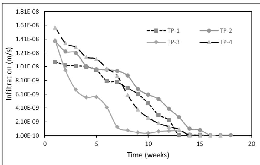
**Fig. 6.** Infiltration rates at Test pads during the first set of measurements.
