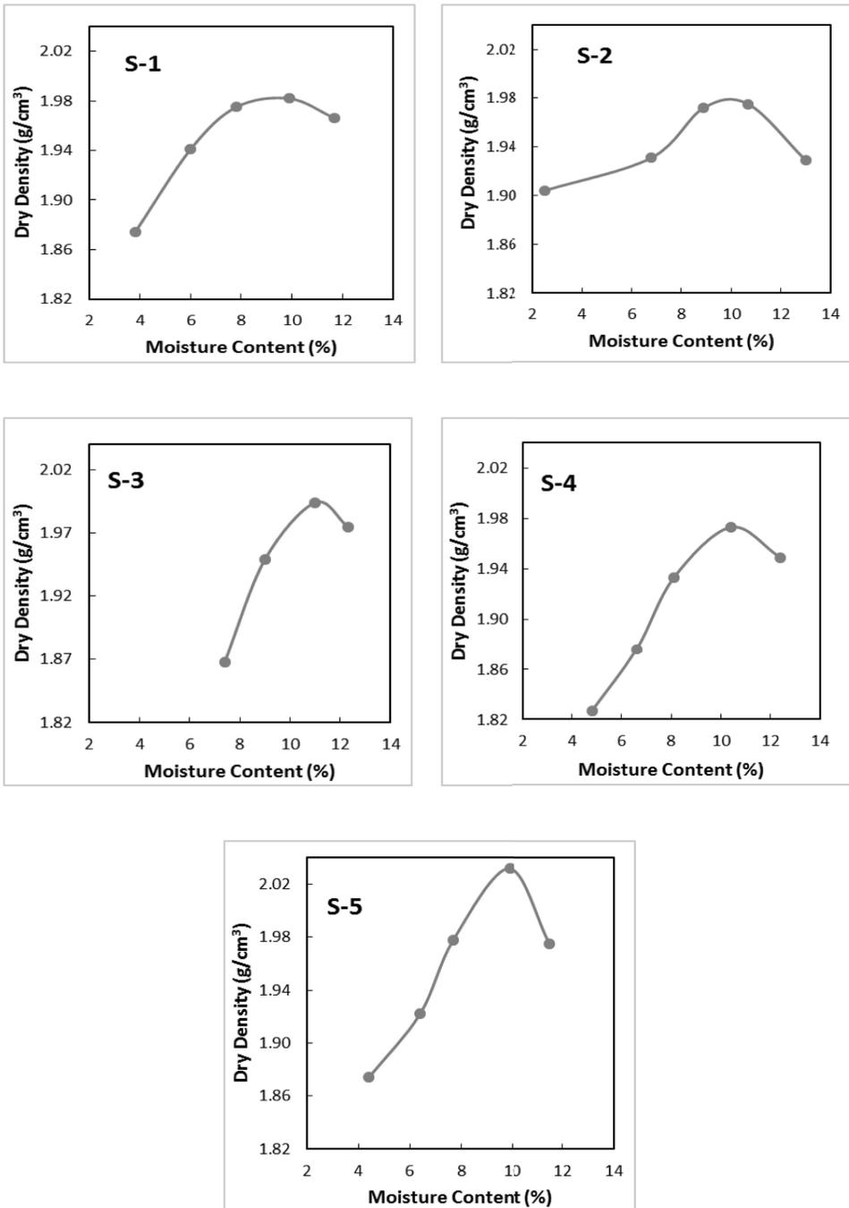
Fig. 1. Compaction curves of soil samples with Modified Proctor Test.
