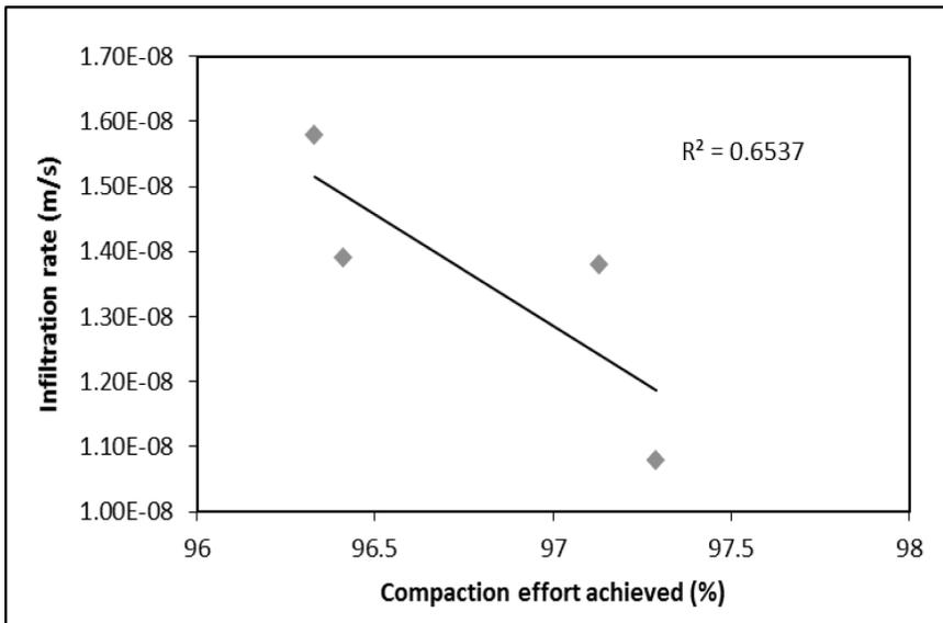
Fig. 7. Relation between compaction effort and infiltration rate during the 1<sup>st</sup> set.
