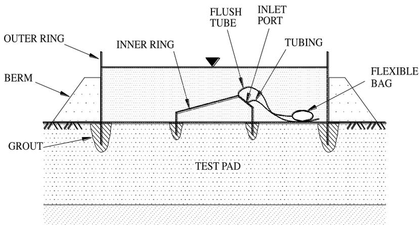
**Fig. 5.** A schematic diagram of the SDRI (adapted from Bozbey and Guler, 2006)
