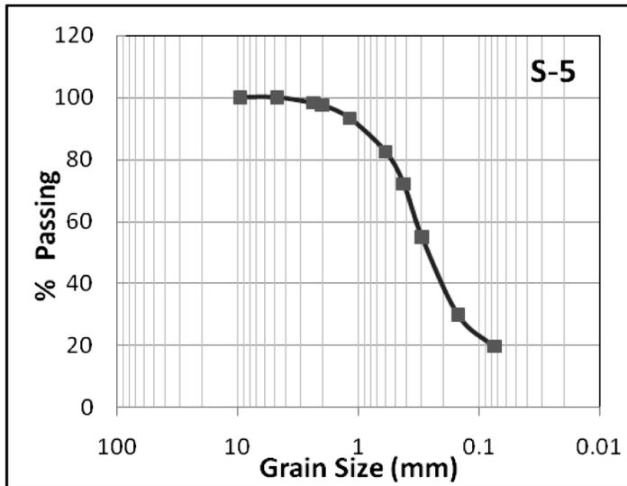
Fig. 2. Particle-size distribution curve for the soil used to construct the test pads.
