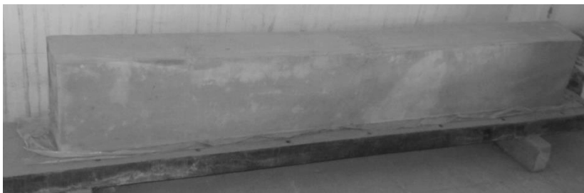
Fig. 5. The beam without drying shrinkage cracks.
