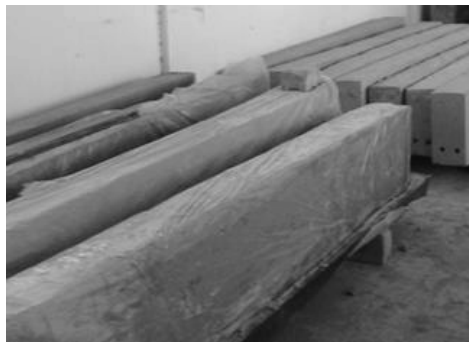
Fig. 4. The beams were covered with plastic sheet in order to decrease evaporation of moisture. The circles in the bottom portion of the beams indicate perforations that are made for tensile reinforcement to be provided after drying and baking.
