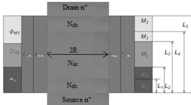
Figure 2. Schematic View of cylindrical DH-DD-TM-SG MOSFET.
