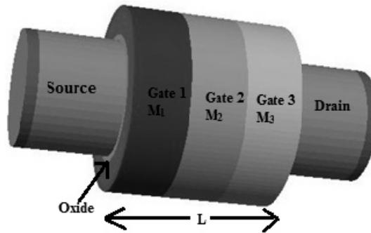
Figure 1. 3D View of cylindrical DH-DD-TM-SG MOSFET.
