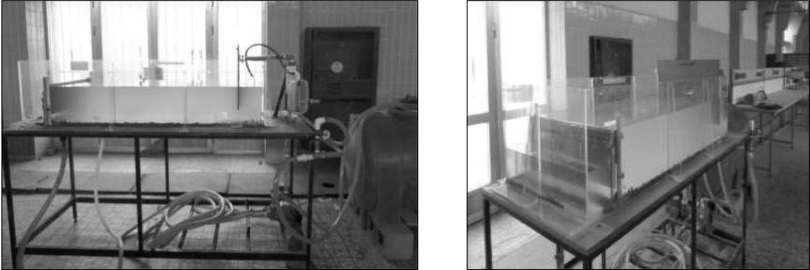
Figure 1. Two perspectives of plain sedimentation rig.
