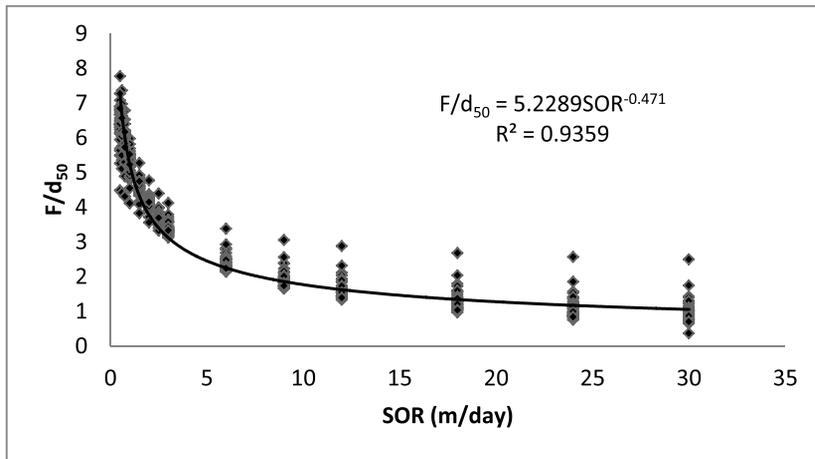
Figure 7. Theoretical efficiency to  $d_{50}$  ratio versus SOR.
