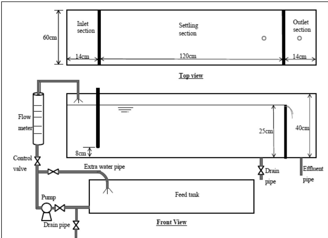
Figure 2. Schematic diagram of plain sedimentation rig.
