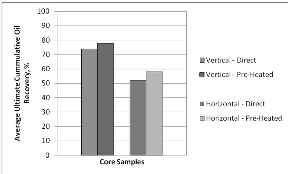
Fig. 9. Average ultimate cumulative oil recovery for all cores.
