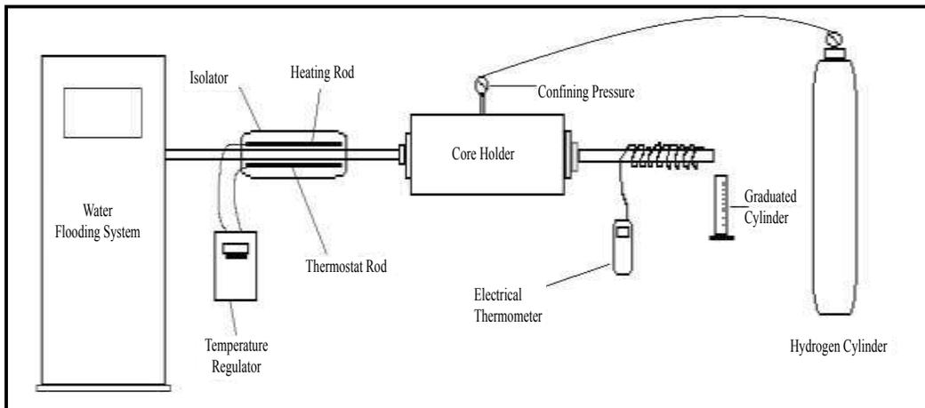
**Fig. 4.** Hot water setup.
