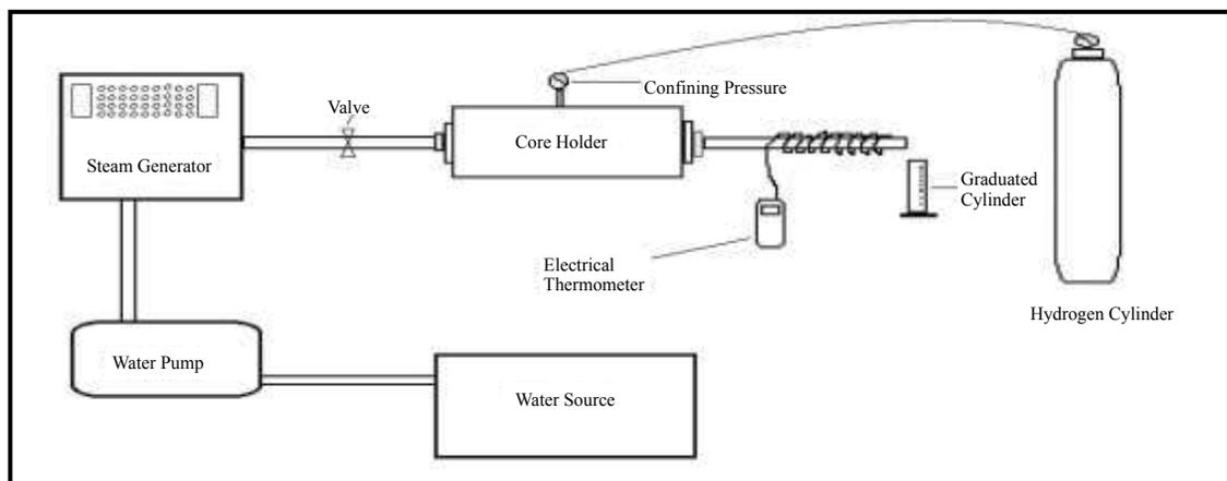
Fig. 5. Steam flooding setup.
