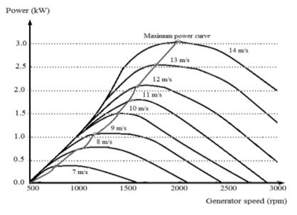
Figure 10. Speed-power curve of a 5 kW wind turbine.
