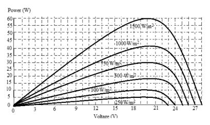
Figure 9. Voltage-power curve of 2 kW solar panels.
