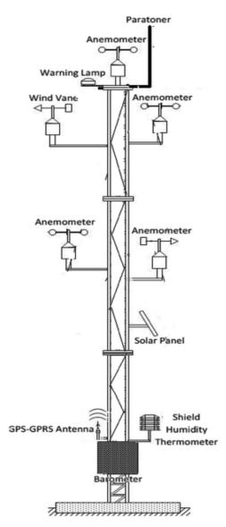
Figure 2. Wind speed/solar radiation measuring station.
