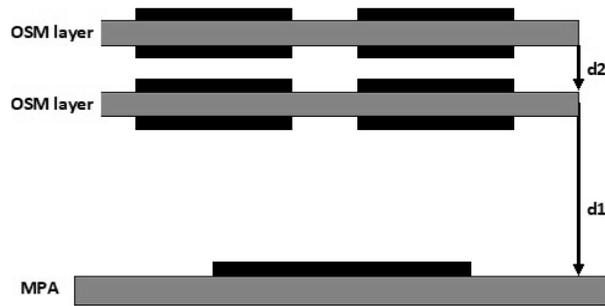
**Figure 13.** Side view of the antenna system with two OSM lens layers.
