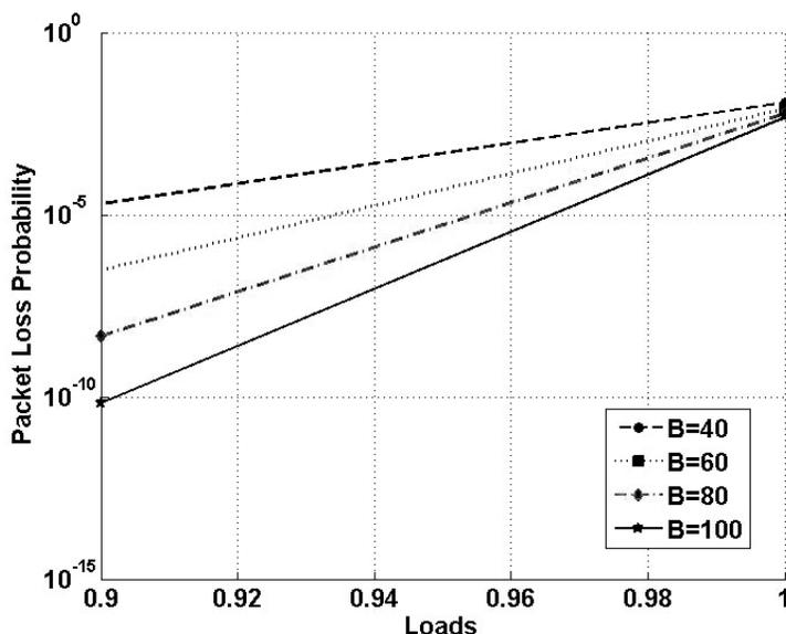
Figure 5. Loss probability vs load under various buffer combinations (S2).
