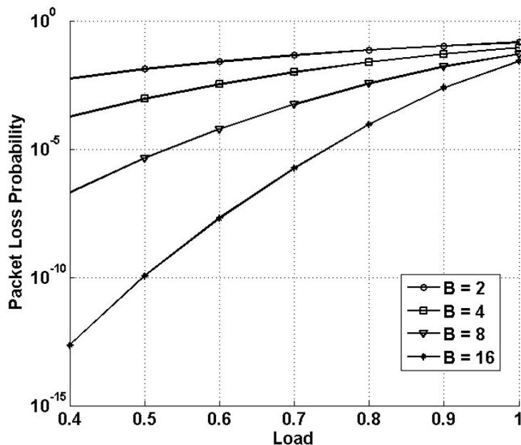
Figure 4. Loss probability vs load under various buffer combinations (S1).
