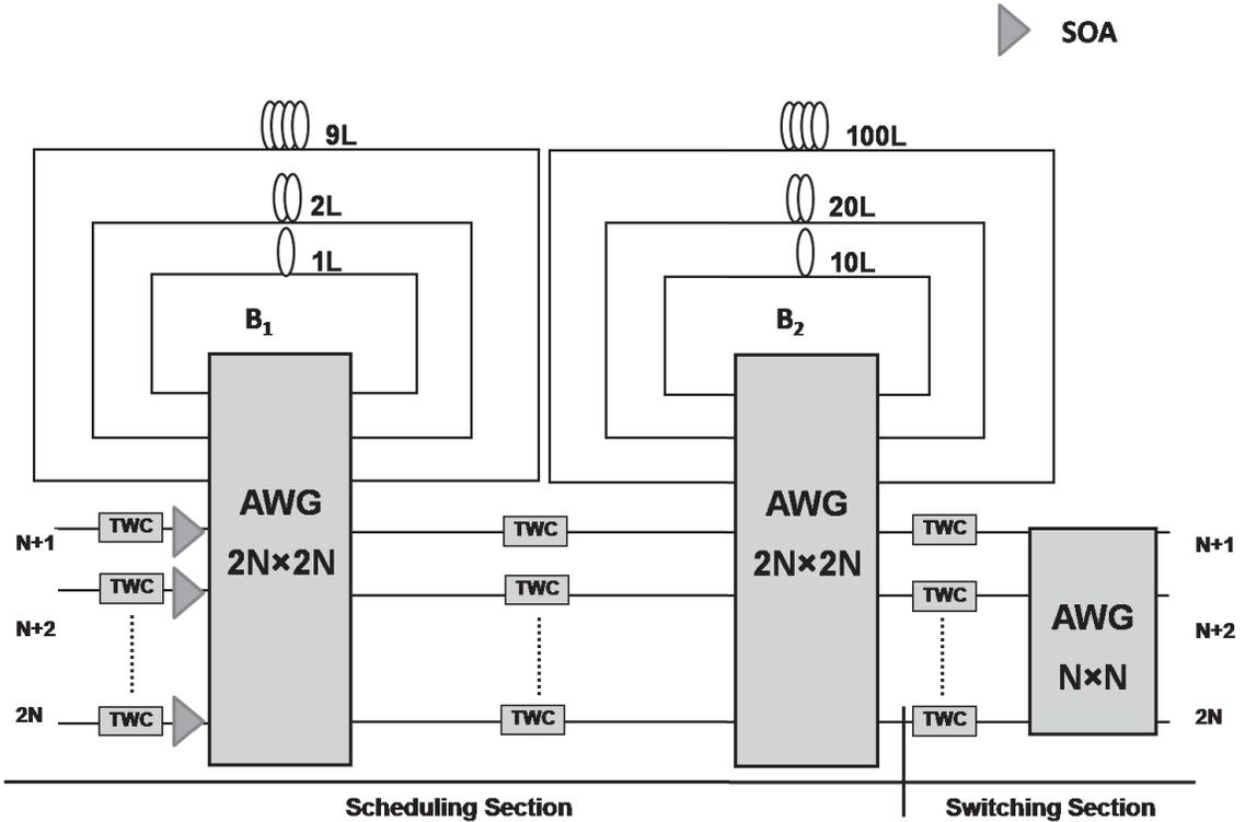
Figure 2. Proposed Design of AWG based Switch (S2).
