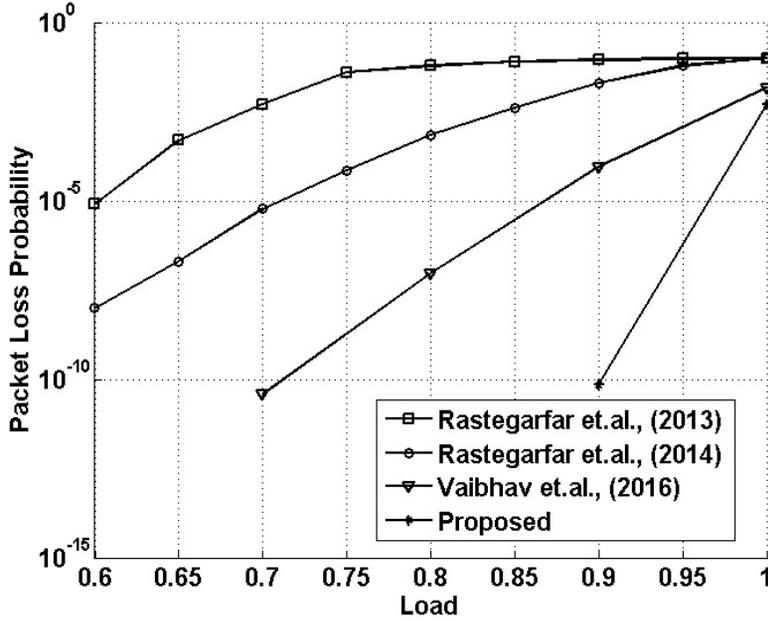
Figure 6. Comparison of recent switch designs in terms of packet loss probability.
