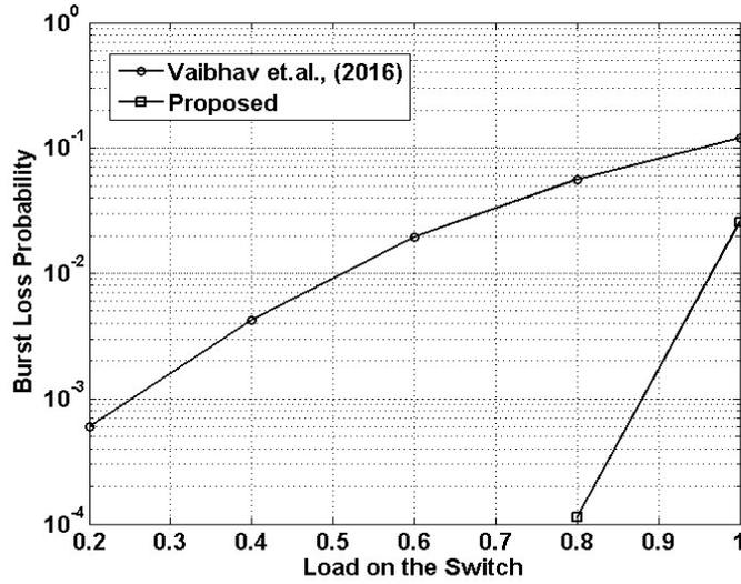
Figure 7. Comparison of recent switch designs in terms of packet loss probability.
