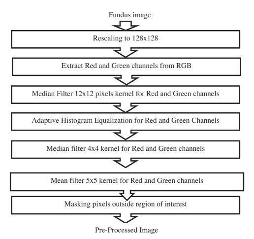
Fig. 3. Series of steps used in the pre-processing.
