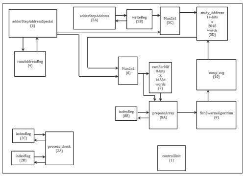
Fig. 7. The datapath of the proposed design.
