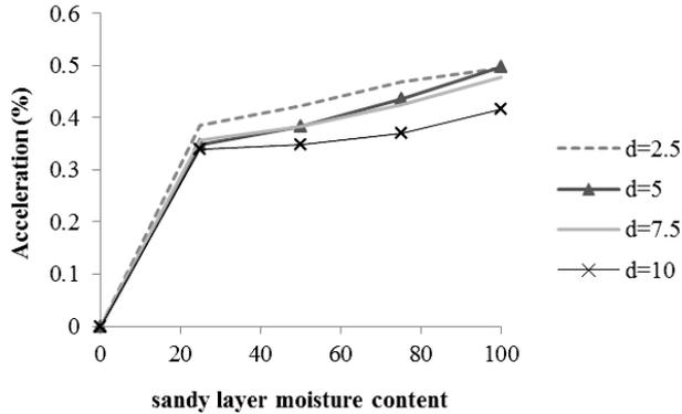
Fig. 16. Acceleration reduction percent versus sandy layer moisture content
