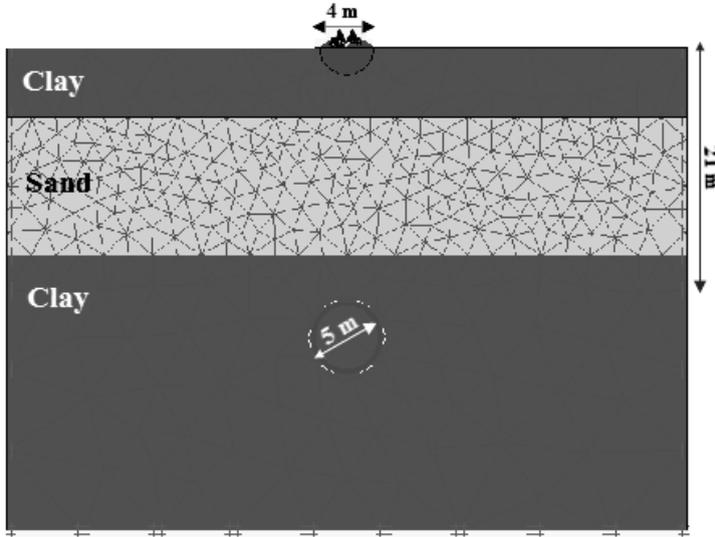
Fig. 1. Numerical model (geometry and boundary conditions)
