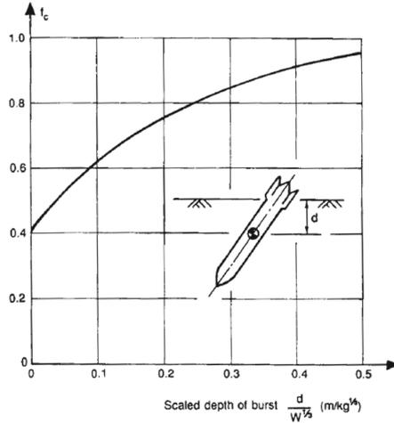
Fig. 2. Dependence of coupling factor on scaled depth of burst (Schmidt & Holsapple, 1980)
