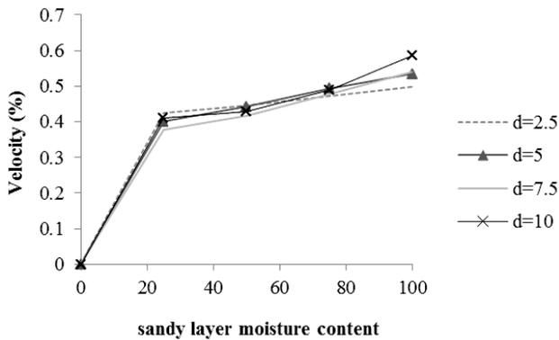
Fig. 15. Velocity reduction percent versus sandy layer moisture content
