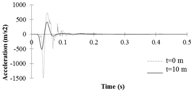
Fig. 8. Acceleration time history versus sandy layer thickness
