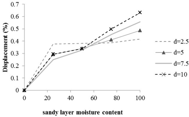
Fig. 14. Displacement reduction percent versus sandy layer moisture content
