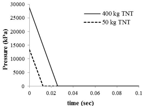
**Fig. 3.** Explosion loading chart for verification analysis
