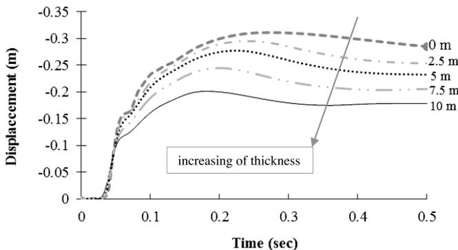
Fig. 6. Displacement time history versus sandy layer thickness
