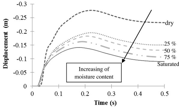
Fig. 11. Displacement time history versus sandy layer moisture content
