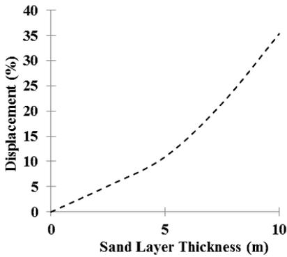
Fig. 9. Displacement reduction percent versus sand layer thickness
