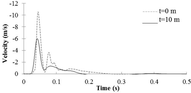
Fig. 7. Velocity time history versus sandy layer thickness
