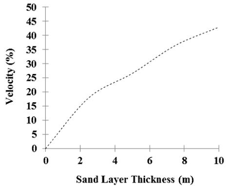
Fig. 10. Velocity reduction percent versus sand layer thickness
