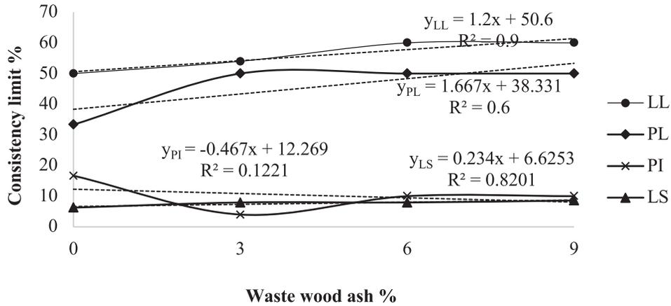
\*LL= Liquid Limit, PL= Plastic Limit, PI= Plastic Index, LS= Linear Shrinkage
