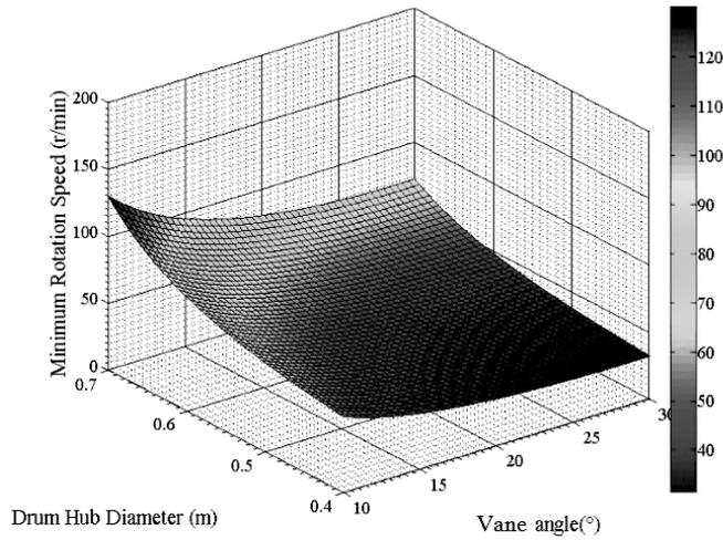
Fig. 4. Relationship of minimum rotating speed with vane angle and drum hub diameter.
