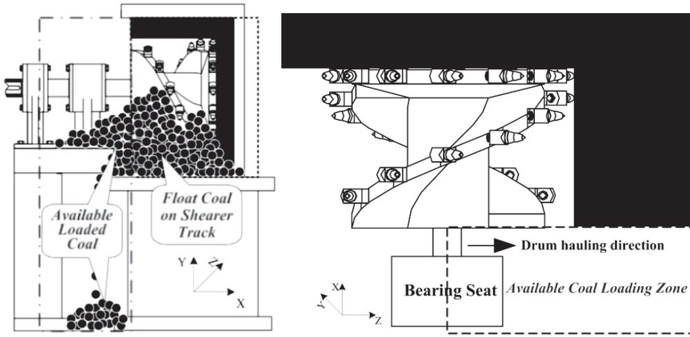
Fig. 10. Scheme of available coal loading zone.
