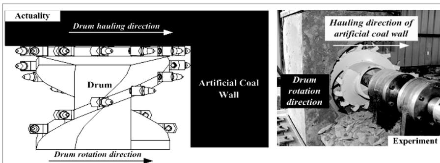
(b) Coal loading in down cutting mode
