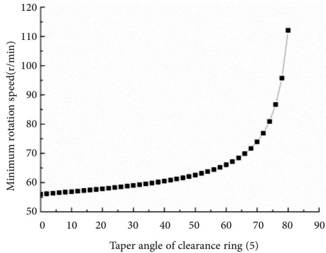
**Fig. 8.** Influence of clearance ring taper angle on drum minimum rotating speed.
