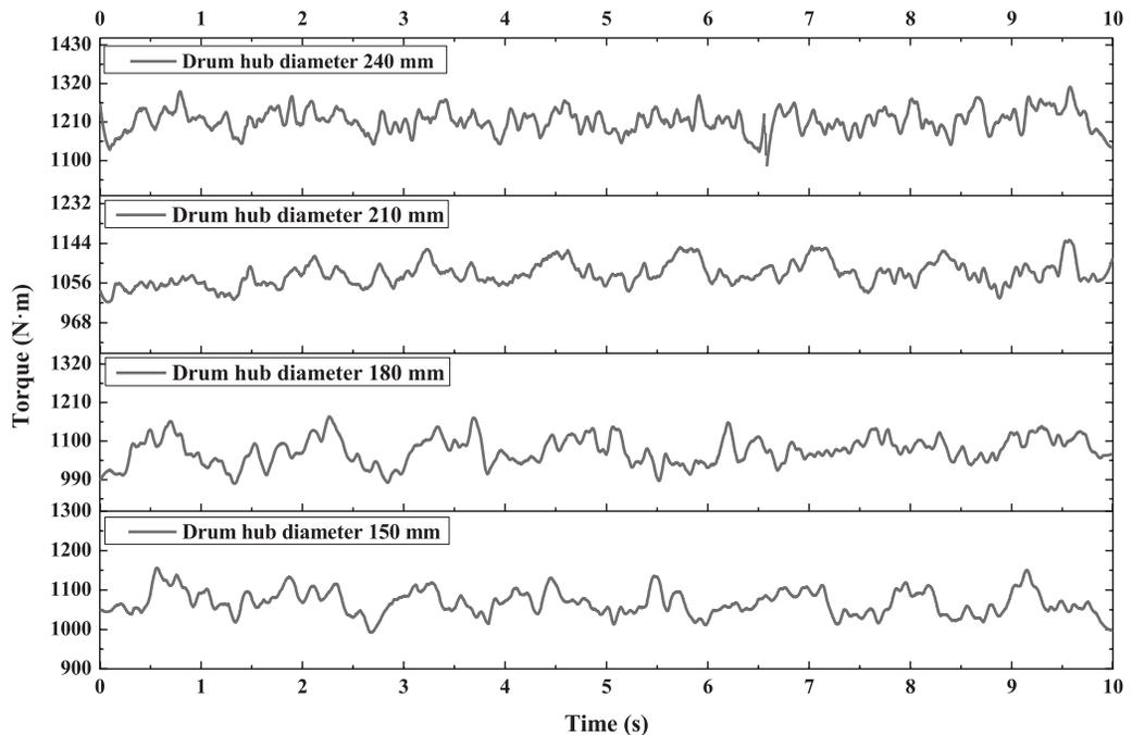
Fig. 13. Torques of four different hub diameter drums (coal loading in drum up cutting mode).
