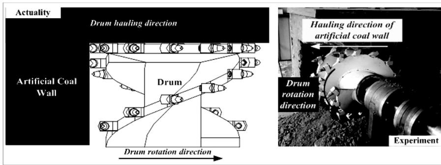
(a) Coal loading in up cutting mode
