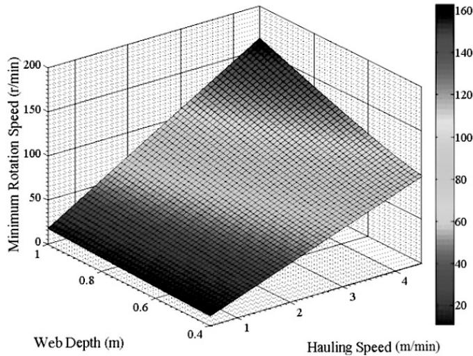
Fig. 7. Relationship of minimum rotating speed with drum hauling speed and web depth.
