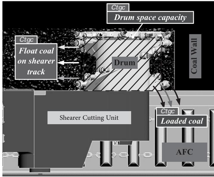
Fig. 2. Work condition of shearer drum.
