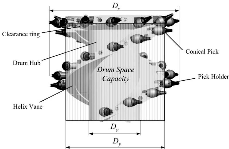
**Fig. 1.** Structure of shearer drum.
