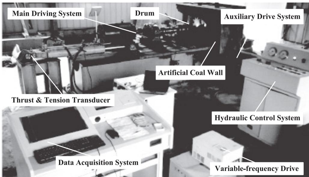
**Fig.9.** Cutting test bed.
