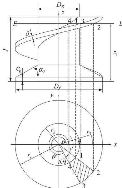
Fig. 3. Section of single helix vane drum.
