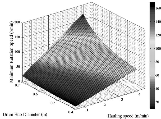
Fig. 5. Relationship of minimum rotating speed with drum hauling speed and drum hub diameter.
