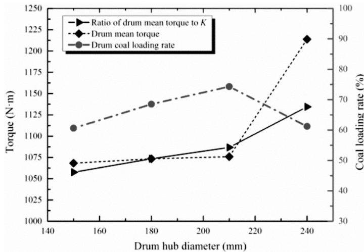
**Fig. 14.** Influence of drum hub diameter on drum torque and coal loading rate (coal loading in drum up cutting mode).
