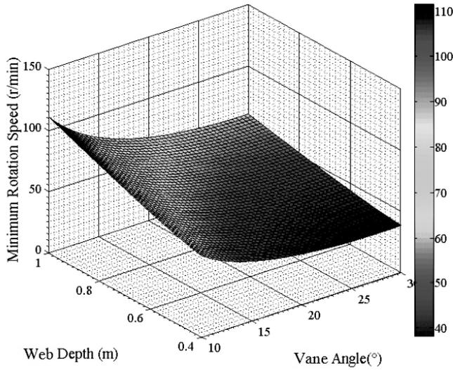
Fig. 6. Relationship of minimum rotating speed with vane angle and web depth.
