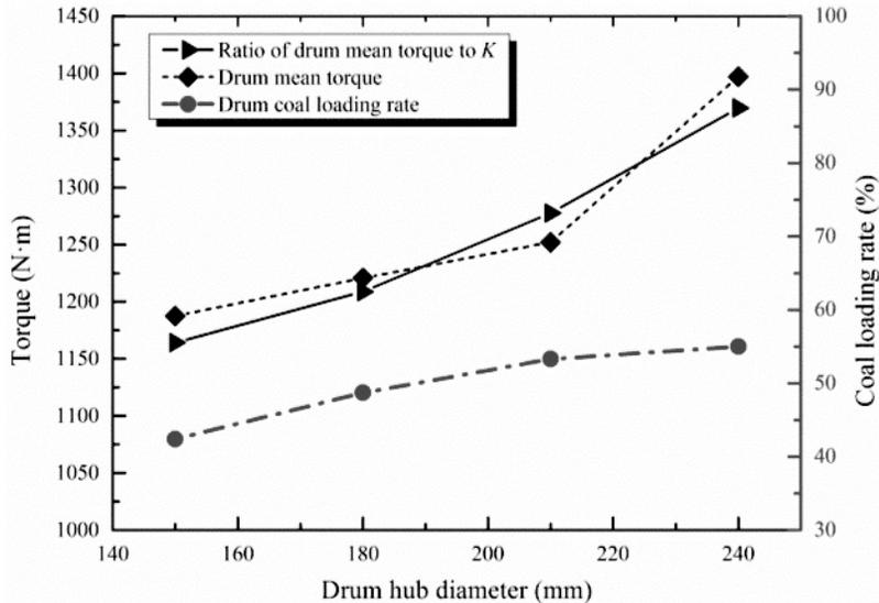
**Fig. 15.** Influence of drum rub diameter on drum torque and coal loading rate (coal loading in drum down cutting mode).
