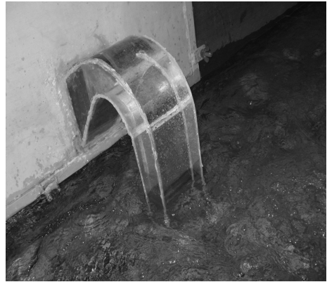
Fig. 9b. Full siphonic discharge
