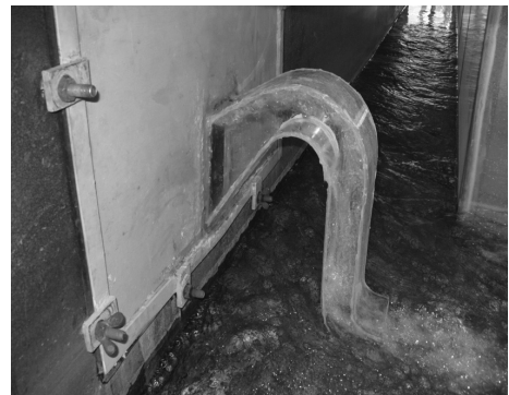
Fig. 8b. Priming siphon
