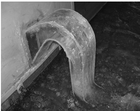
Fig. 8b. Priming siphon
