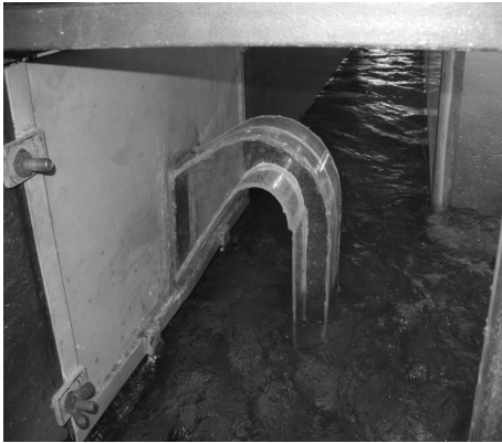
Fig. 9b. Full siphonic discharge
