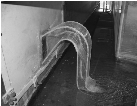
Fig. 8a. The beginning of priming siphon
