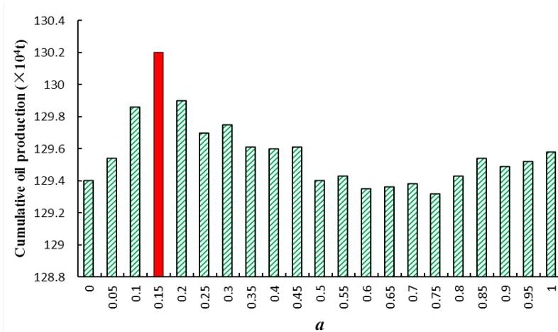
Fig. 5. Cumulative oil productions of cases with different values of  $a$
