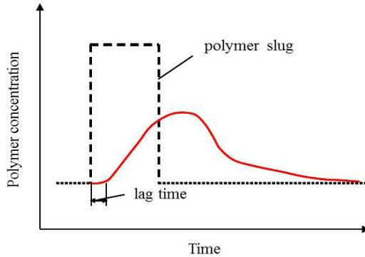
**Fig. 4.** Schematic plot of polymer concentration curve of the production well
