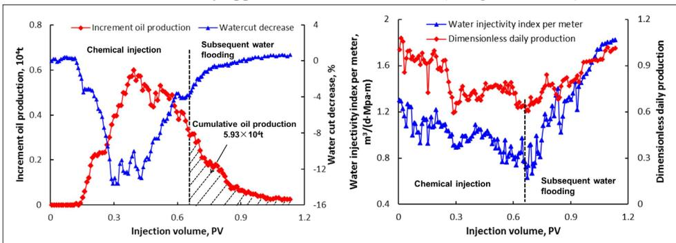
(a) Watercut and incremental oil production (b) Injectivity index and liquid production
