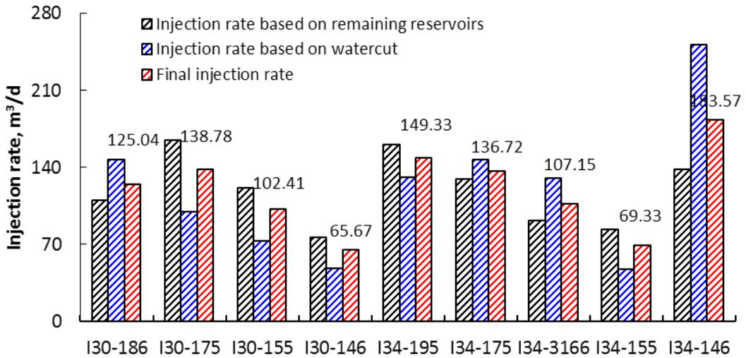
Fig. 7. Final allocation result both considering reserves and watercuts ( $\alpha=0.6$ )
