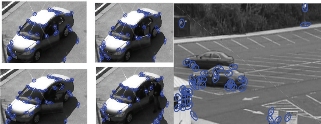
Fig. 4. Computation of salient points using 3D Cuboid Detector
