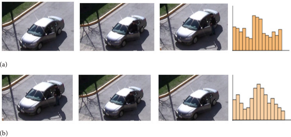
Fig. 3 (a) & (b). Shows BoW representation based on our approach. Our approach differentiated getting into the car and getting out of the car as the different interactions with different histograms
