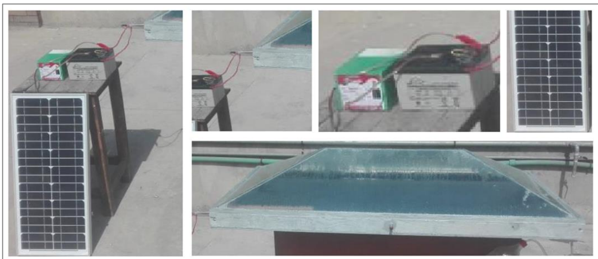
Figure 3. Physical model of pyramid solar water desalination unit with EWH.
