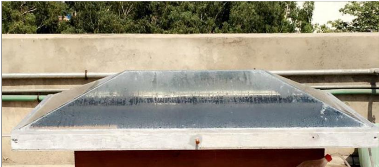
Figure 2. Physical model of pyramid solar water desalination unit
