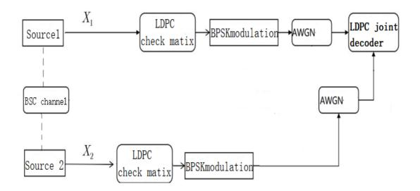
Figure 1. The diagram of distributed source coding Based on memory-less correlated source and Low-Density Parity-Check Code.
