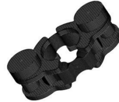
Figure 7. The structure of the cycloid rotor pump. Figure 8. Mesh on internal flow field.
