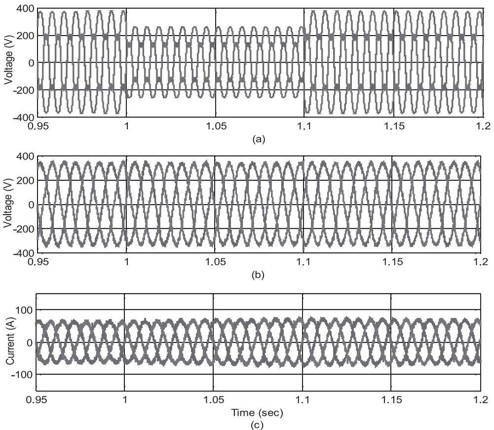
**Figure 12.** Compensation during voltage sag (a) supply voltage (b) load voltage and (c) supply currents.
