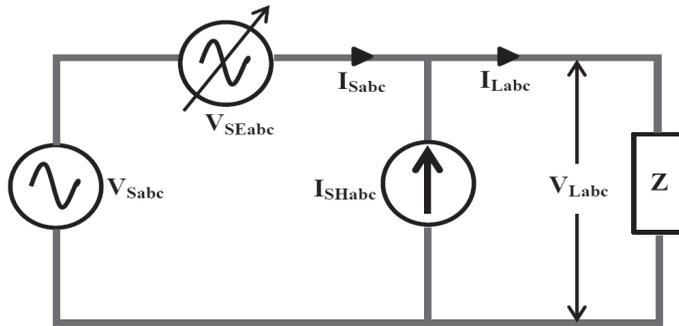
Figure 2. Equivalent circuit of UPQC.
