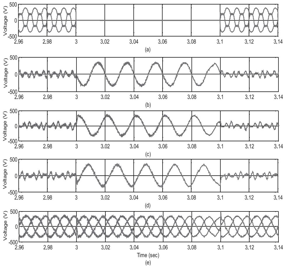
**Figure 16.** (a) Supply voltage (b) injected voltage in phase A (c) injected voltage in phase B (d) injected voltage in phase C and (e) load voltage.
