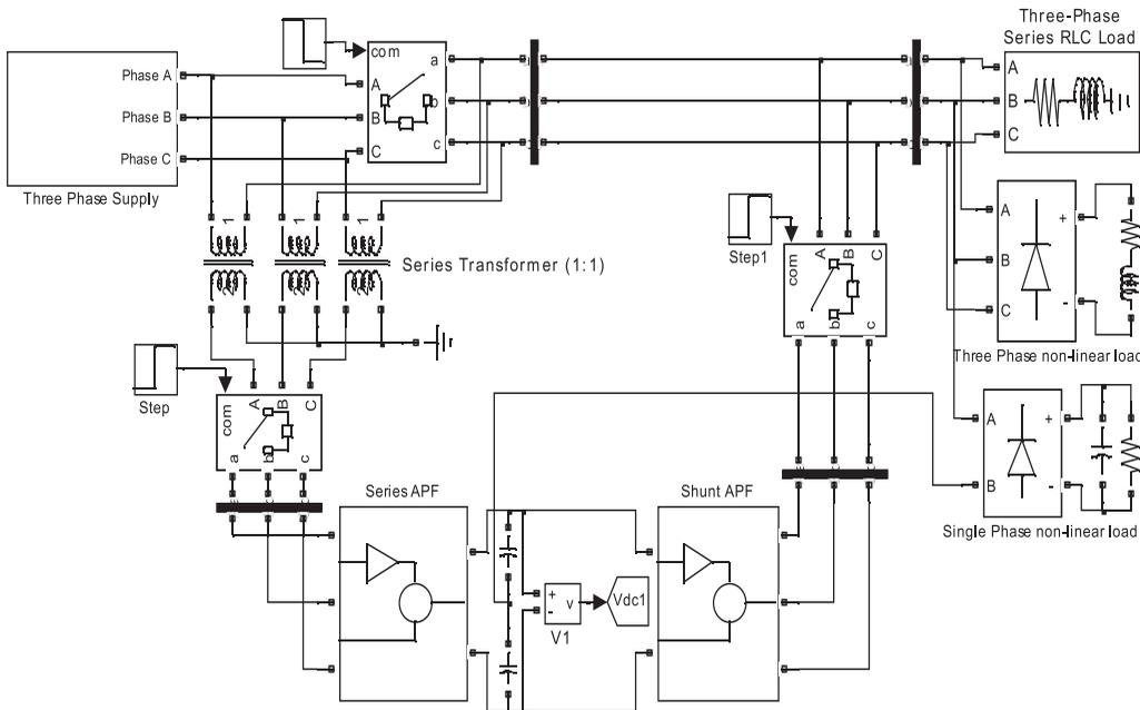
Figure 8. UPQC Matlab/Simulink model of three-phase four-wire system.
