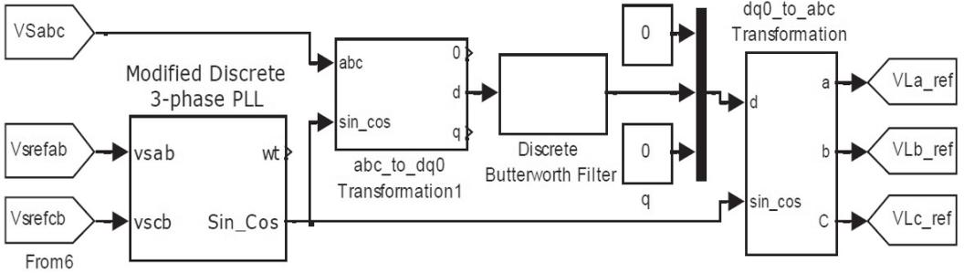
Figure 6. Series controller using SRF.
