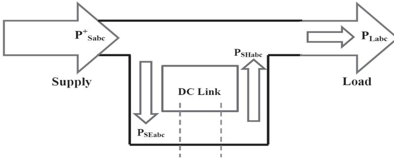
Figure 5. Active power flow during voltage swell conditions
