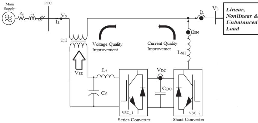
Figure 1. Basic configuration of UPQC.
