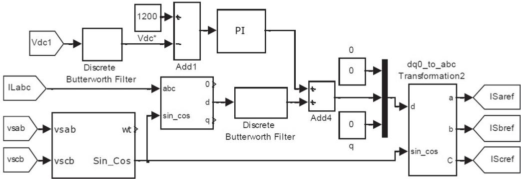
Figure 7. Shunt controller using SRF
