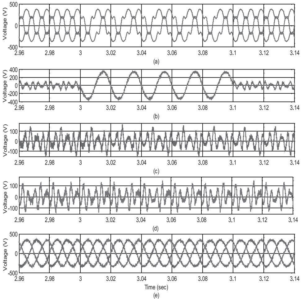
**Figure 15.** (a) Supply voltage (b) injected voltage in phase A (c) injected voltage in phase B (d) injected voltage in phase C and (e) load voltage.
