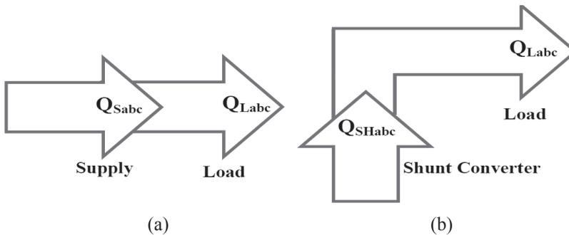
Figure 3. Reactive power flow (a) without UPQC (b) with shunt converter
