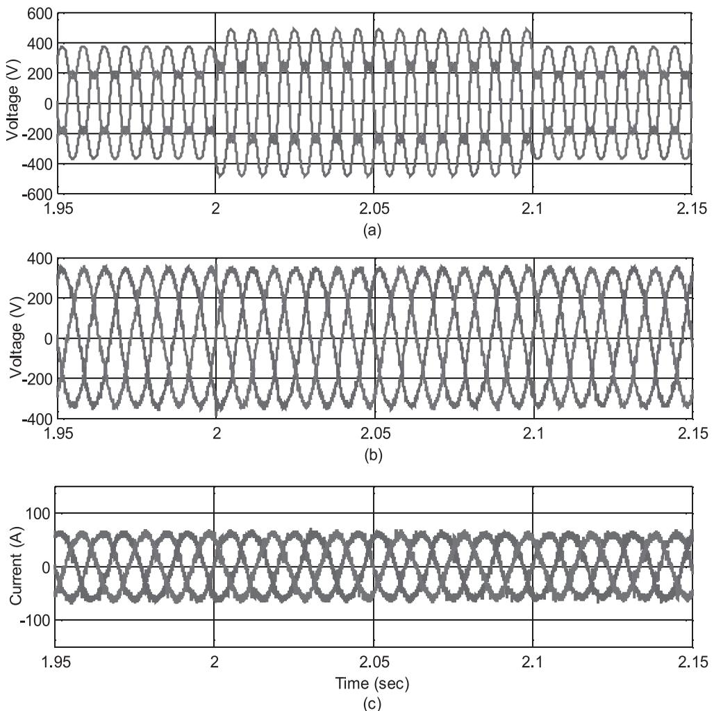
**Figure 13.** Compensation during voltage swells (a) supply voltage (b) load voltage and (c) supply currents.
