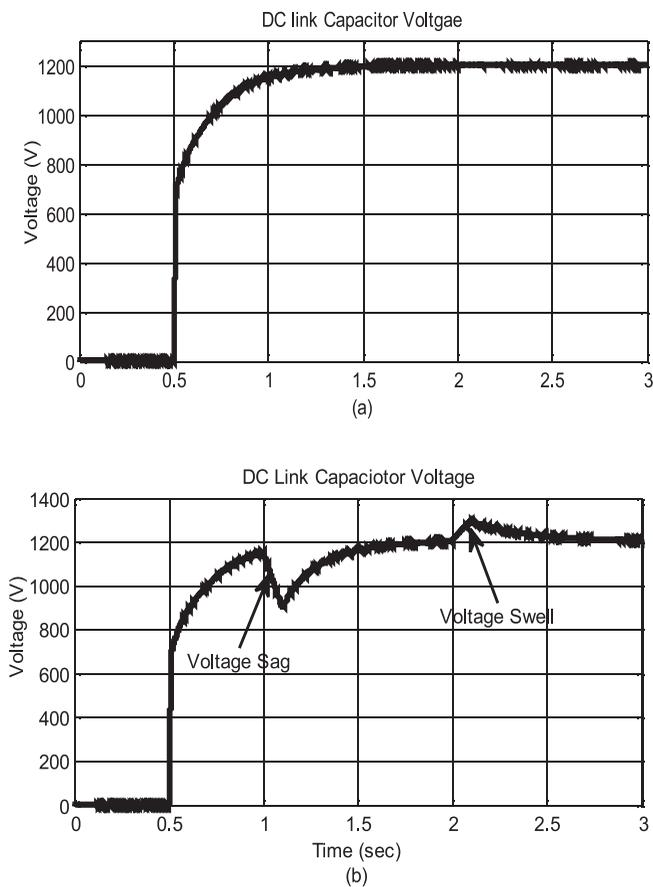
**Figure 14.** Capacitor voltage during (a) normal conditions and (b) voltage sag/swell.
