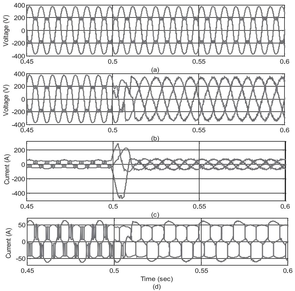
**Figure 9.** Compensation of (a) supply voltage, (b) load voltage, (c) supply currents, and (d) load current.
