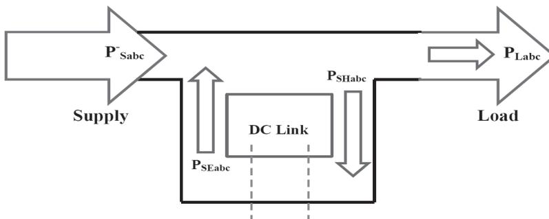
Figure 4. Active power flow during voltage sag conditions
