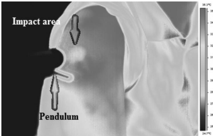
**Fig. 2.** Thermal image showing the measured impacted area. (Alkhaledi, 2010)
