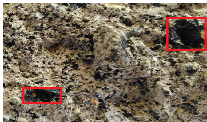
Figure 1. Different distribution regions of bitumen in the briquette internal structure
