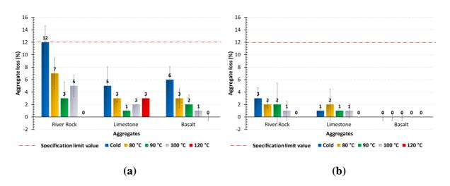
Figure 2. Vialit adhesion test results; (a) B50/70 binder with 1% PPA, (b) B160/220 binder with 1.1% PPA.
