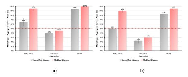
Figure 3. Nicholson stripping test results; a) B50/70 binder, b) B160/220 binder.
