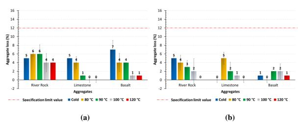
Figure 1. Vialit adhesion test results (a) unmodified B50/70, (b) unmodified B160/220
