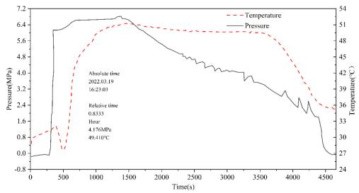
Figure 3 Pressure variation of the gas well when it starts to produce gas
