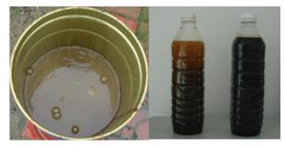
Figure 4 Liquid samples lifted out from the gas well
