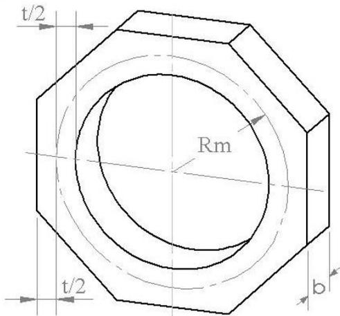
Figure 1(b): Dimensions of a deforming ring
