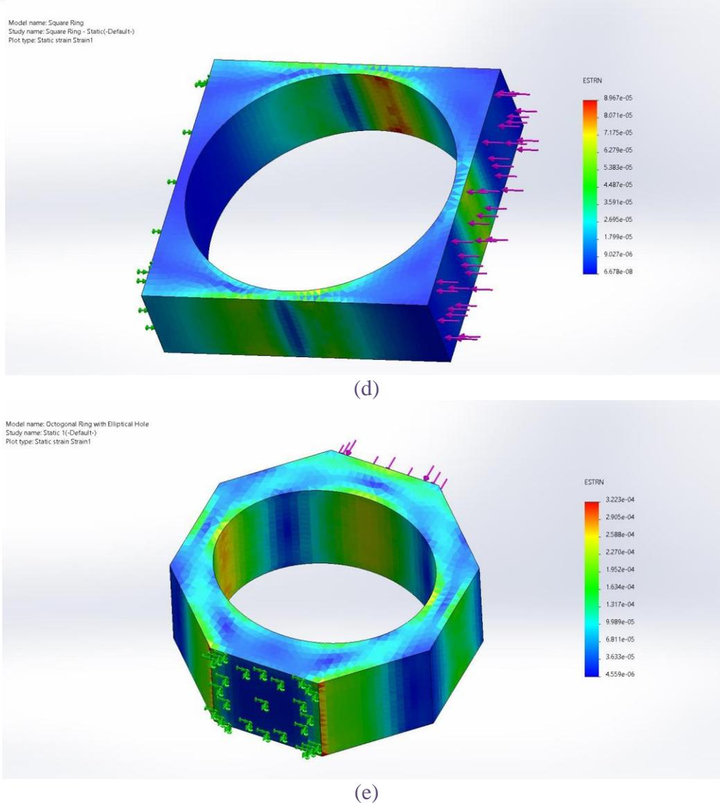
Figure 4 (a - e): The resulting strain on applying SOLIDWORKS finite element analysis on deforming ring models under this study.
