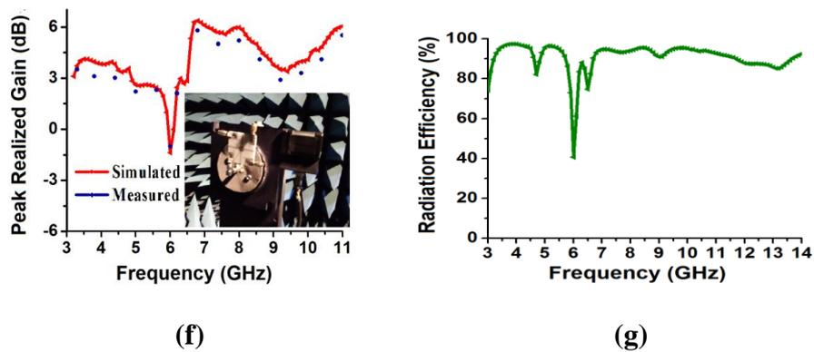
The 3D Radiation pattern of the four-port MIMO antenna is depicted in Fig. 3(d) at 3.6 GHz and in Fig. 3(e) at 6.6 GHz. The realized gain varies from 4 dB to 6.3 dB as shown by Fig. 3(f). The realized radiation efficiency of the MIMO antenna is greater than 90% in the lower operating band and greater than 85% in the upper-frequency band and drops down at the notch band as demonstrated by Fig. 3(g).
