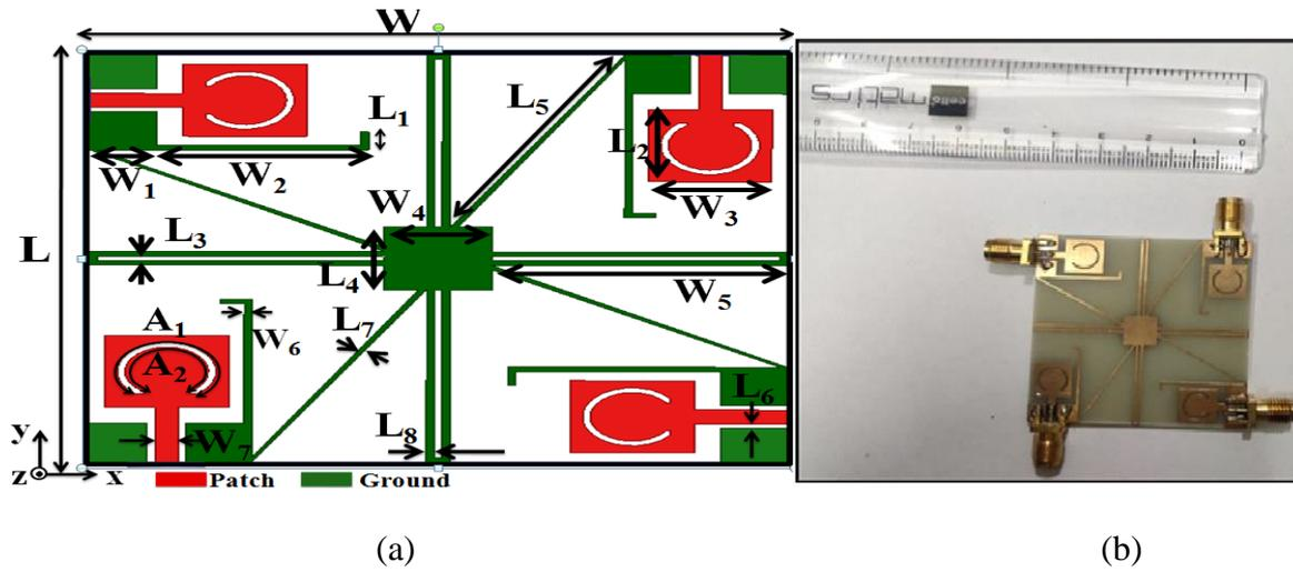
**Figure 1**(a) Proposed CPW fed four elements CSRR based antenna (b) Proposed hardware of prototype
