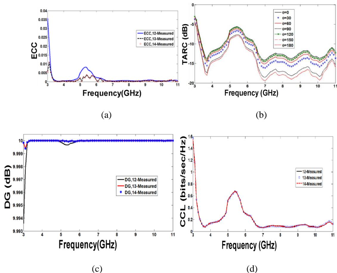
**Figure 4** Parameters of measured prototype (a) ECC (b) TARC (c) DG (d) CCL
