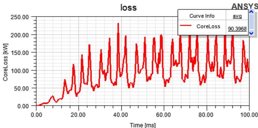
Figure 8. Core loss curve
