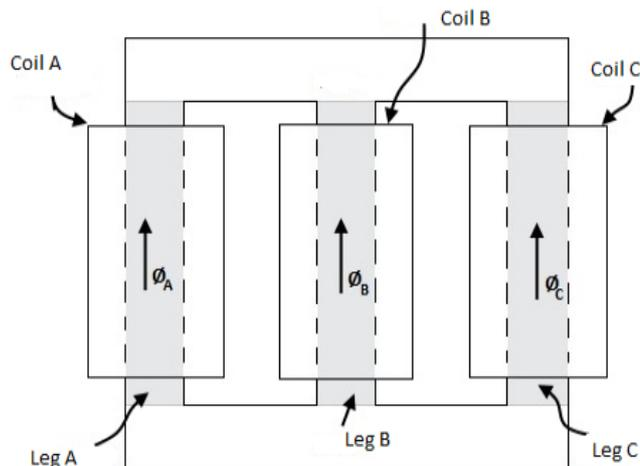
**Figure 4.** Basic structure of 3-legged shunt reactor core.
