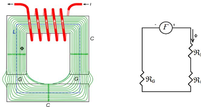
**Figure 3.** Electromagnet with air gap and magnetic circuit equivalent
