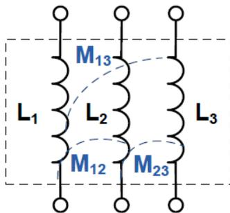
Figure 2: Winding model of three phase reactor [8].
