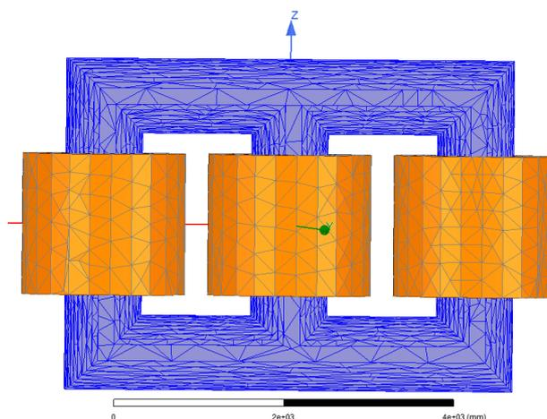
**Figure 5.** Structure of designed shunt reactor and mesh.
