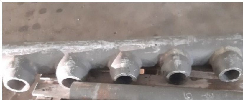
Figure 1. Outlet manifold bottom header.
