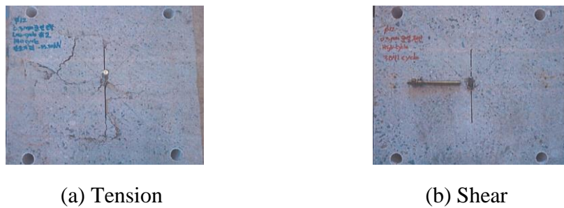
Figure 9. Simulated seismic tension and shear test failure shape
