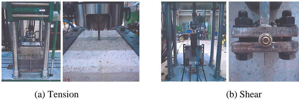
Figure 6. Tension and shear test setup
