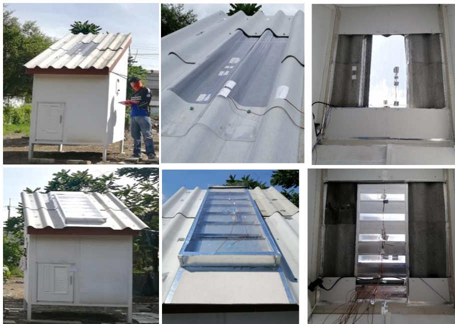
Figure 4. Photographs of the typical house (top) and Skylight Solar Chimney House (bottom).
