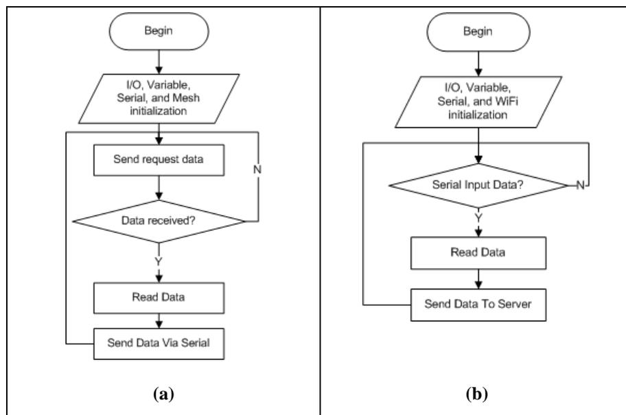
**Figure 3** Flowchart (a) Server Mesh and (b) Gateway
