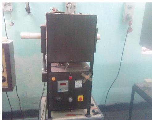
**Fig. 2.** Electrically heated tubular furnace
