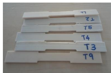
Figure 8. Tensile test specimen before testing
