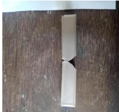
Figure 14. Impact Strength Tested Specimen
