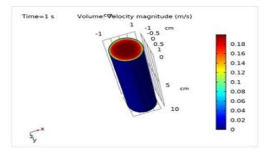
speeds as the center of the pipe is approached is shown in figure 5.
