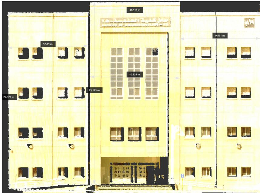
Figure 6: The point cloud dimensions captured by Autodesk ReCap Software[\*]
