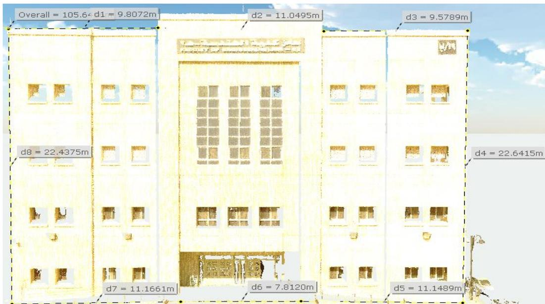
Figure 7: The point cloud dimensions captured by Faro Scene Software [\*\*]
