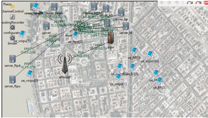
Figure 6.: SimuLTE scenario representing LTE-A network.
