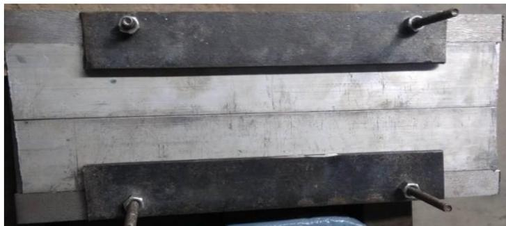
**Figure 3.** Clamping of Al strip on cast iron bed
