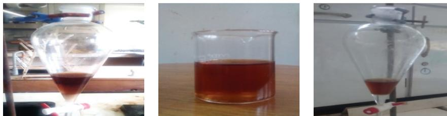
**Figure 1.** Phase separation and purification of biodiesel.
