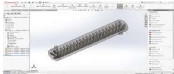
Figure 6. Internal view of 5-Turns of helical tube STHXs
