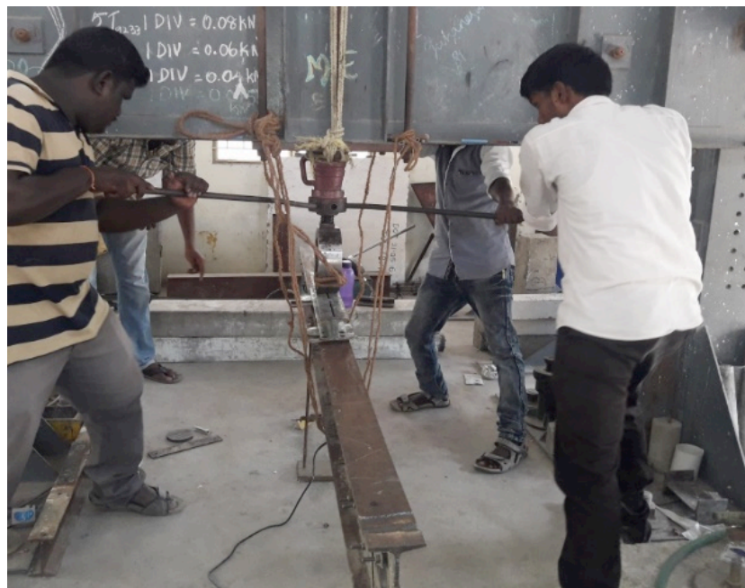
Figure 19 Loading of the castellated beam
