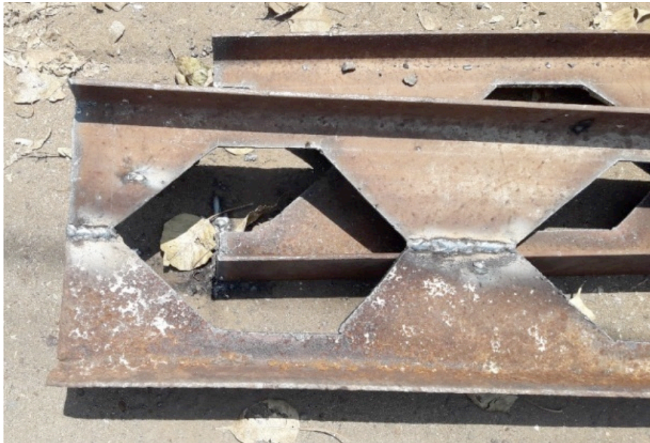
Figure 2 Illustration of the castellated beam
