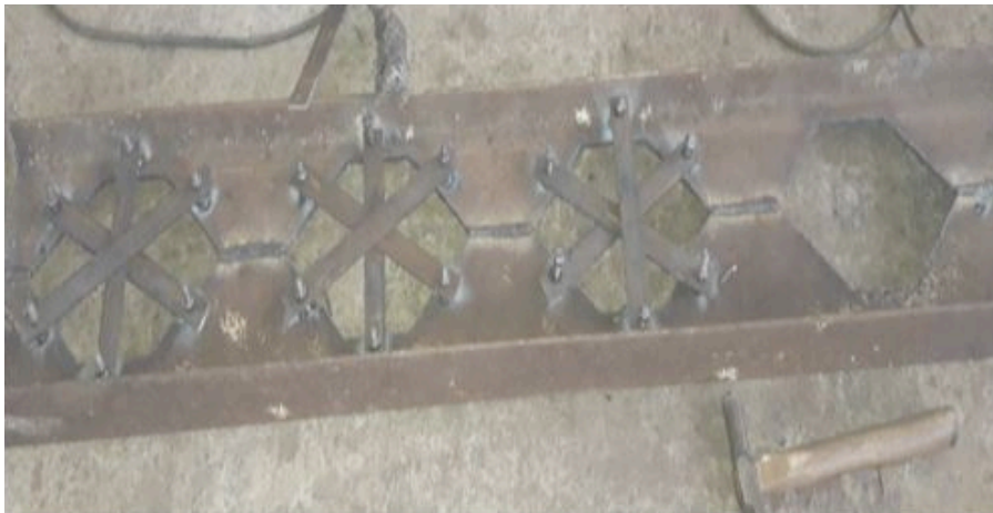
Figure 14 Stiffeners in Castellated Beams Chassis
