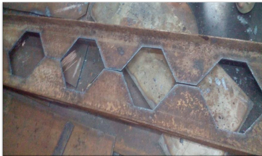
Figure 13 Castellated beam chassis with hexagonal holes
