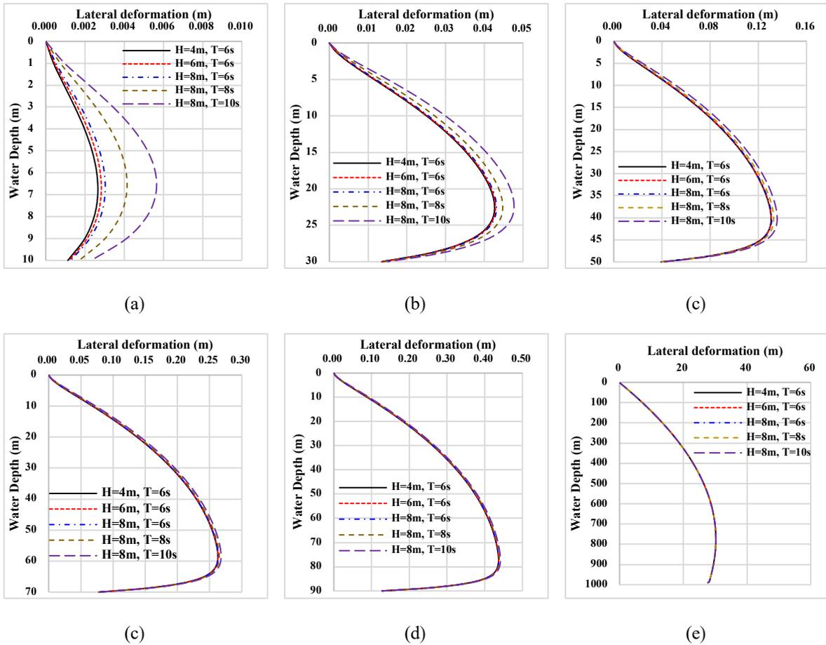
**Figure 5.** Lateral deformations of the pipe under different ocean waves with water depth of (a) 10m, (b) 30m, (c) 50m, (d) 70m, (e) 90m, and (f) 1000m.
