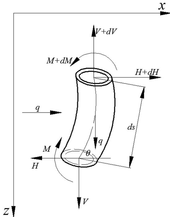
Figure 2. Sketch of a differential drill pipe.
