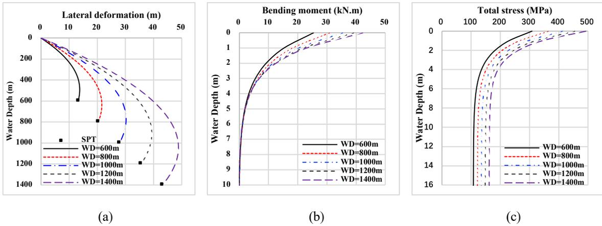
Figure 7. Variation of deformation and mechanical behaviour of pipe with water depth: (a) lateral deformation of drill pipe, (b) bending moment of drill pipe, and (c) total stress of drill pipe.
