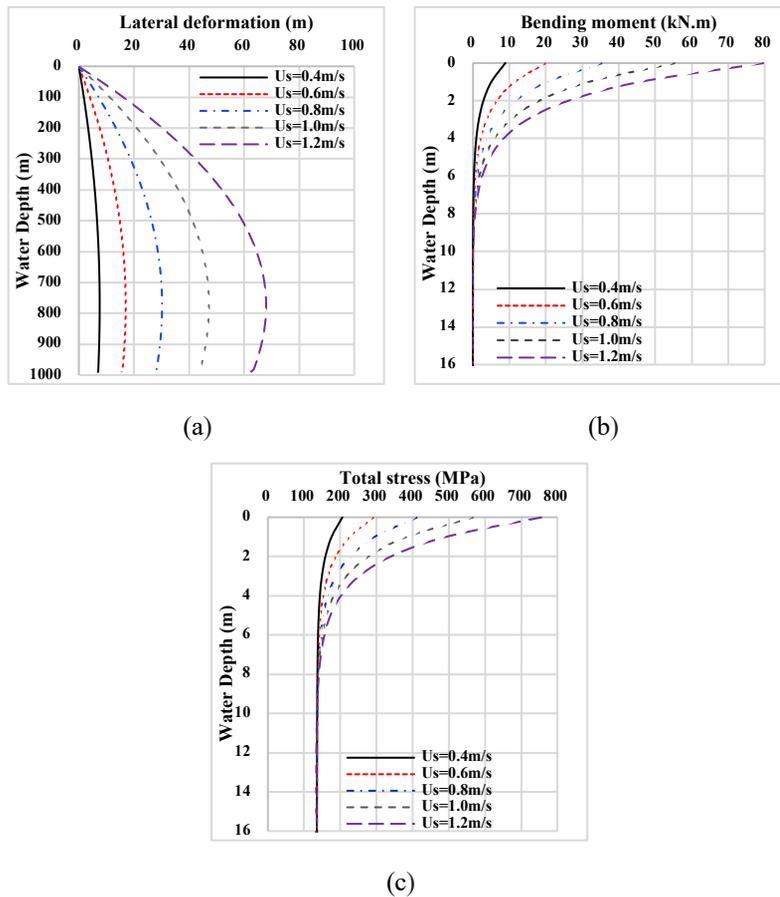
**Figure 6.** Effect of ocean wave on the pipe during SPT installation: (a) lateral deformation of drill pipe, (b) bending moment of drill pipe, and (c) total stress of drill pipe.
