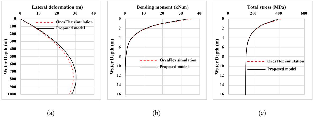
**Figure 4.** Comparisons of the proposed model and OrcaFlex simulation: (a) lateral deformation of drill pipe, (b) bending moment of drill pipe, and (c) total stress of drill pipe.
