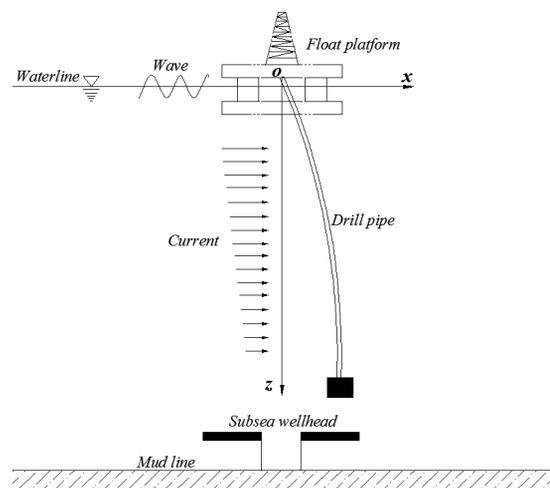
**Figure 1.** Schematic diagram of SPT installation using drill pipe.
