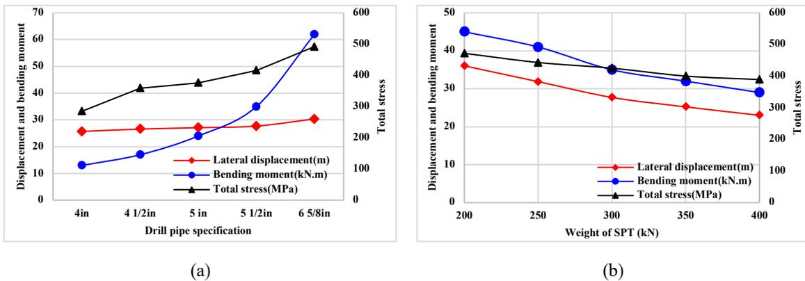
Figure 8. Maximum displacement last node, bending moment, and total stress of drill pipe under (a) different drill pipe specifications and (b) weight of SPT.
