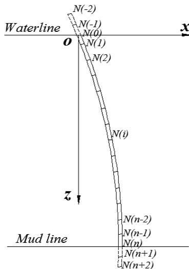
Figure 3. Schematic diagram of drill pipe discretization.
