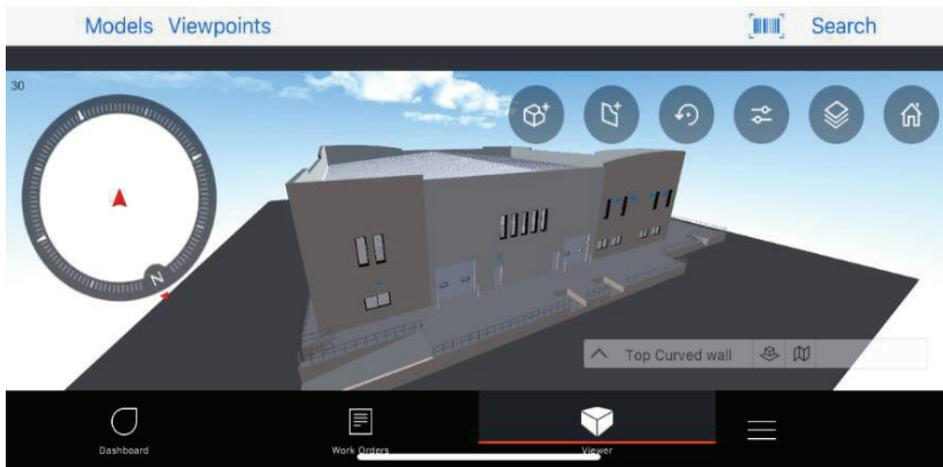
**Figure 12.** Adopted BMS application iOS app user interface: integration of BIM to BMS.
