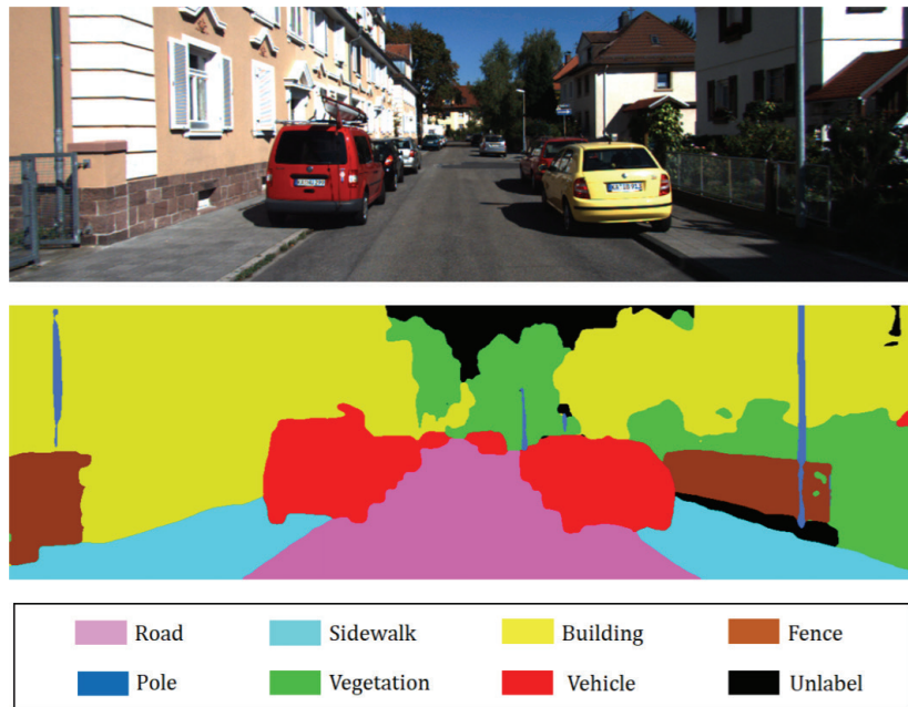
Figure 8. Semantic segmentation with class labels (Jeong et al., 2018).
