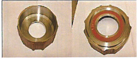
Fig. 6. Diffuser Housing (Material: Cast Iron; Outer dia: 140mm Centre Hole Dia: 60mm)
