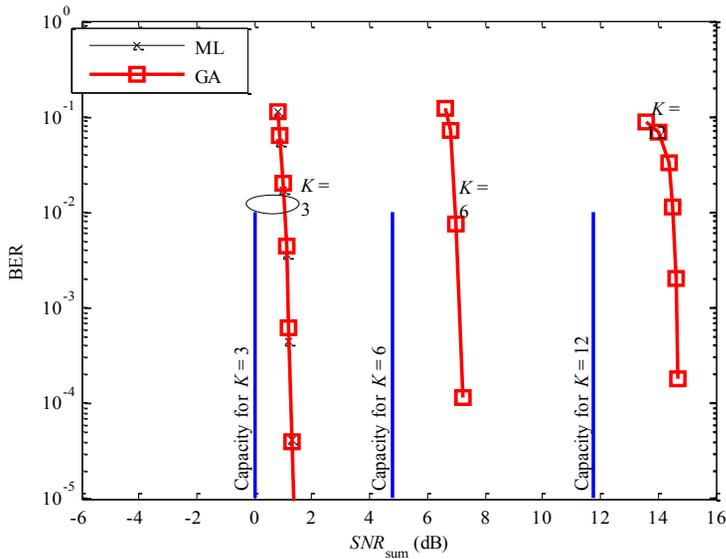
**Figure 8.** IDMA systems with EPC and SPC over AWGN channels. Rate-1/3 turbo coding followed by rate-1/2 repetition coding is used for each user with QPSK modulation [105].
