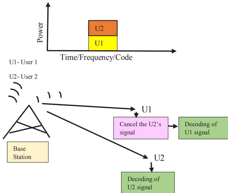
**Figure 3.** Basic NOMA principle in downlink communication with one base station two users.
