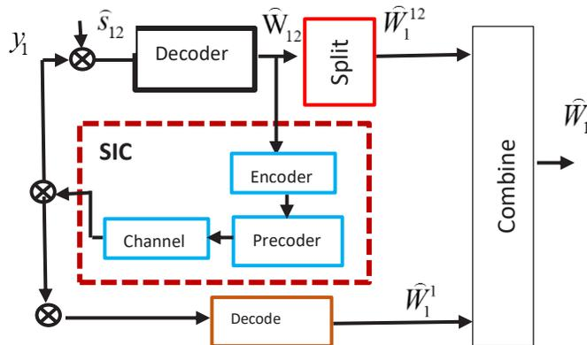
Figure 10. RSMA receiver block for single user.
