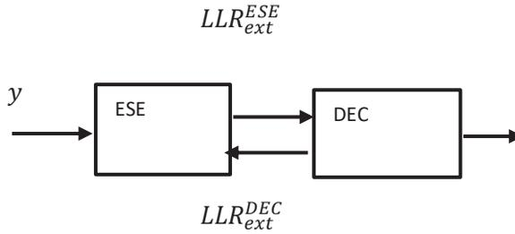
**Figure 7.** Iteration between ESE and DEC in IDMA receiver.
