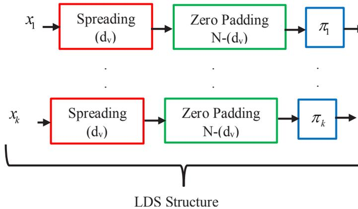
Figure 4. LDS structure for signature sequence generation.
