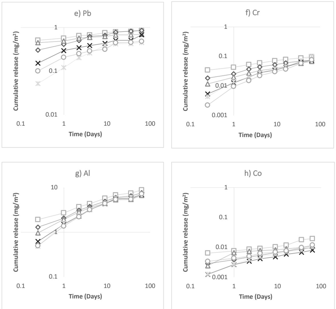
**Figure 2.** Cumulative release of heavy metals leached from the samples up to 64 days as represented in graphs as a) cadmium (Cd); b) copper (Cu); c) zinc (Zn); d) nickel (Ni); e) lead (Pb); f) chromium (Cr); g) aluminium (Al) and; h) Cobalt (Co) leached from the samples respectively.
