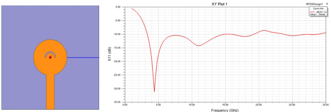
**Figure 4.** Circular patch antenna with half annulus slot: design and results.
