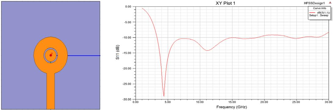
**Figure 5.** Circular patch antenna with an annulus slot: design and results.
