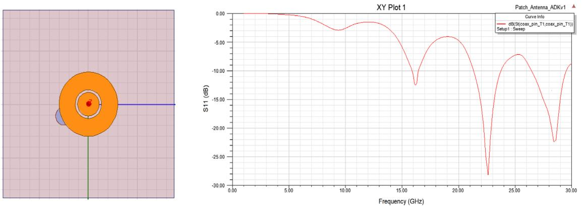
**Figure 10.** Coaxially fed circular antenna with an annulus slot: design and results.
