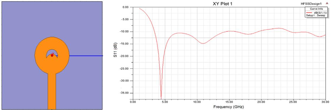
**Figure 3.** Circular patch antenna with a crescent slot: design and results.
