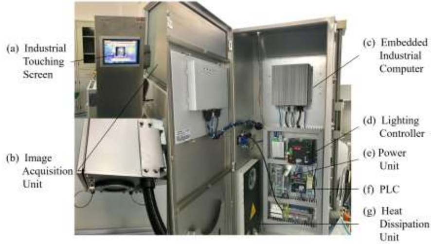
Figure 2. The automatic code recognition system.
