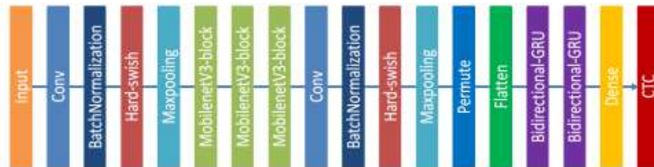
Figure 7. The structure of the modified CRNN model.
