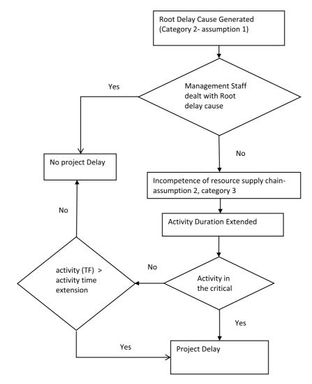
Fig. 3. Project Delay Occurrence (PDO) Model.
